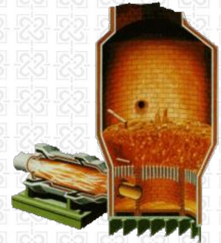
流化床炉 Fluidized Bed Furnace
